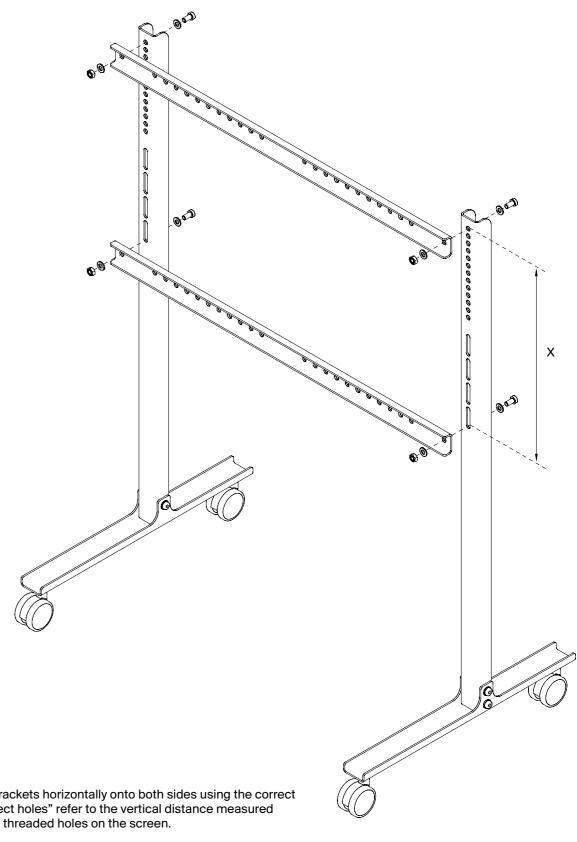
Mount the brackets horizontally onto both sides using the correct holes. "Correct holes" refer to the vertical distance measured between the threaded holes on the screen.
