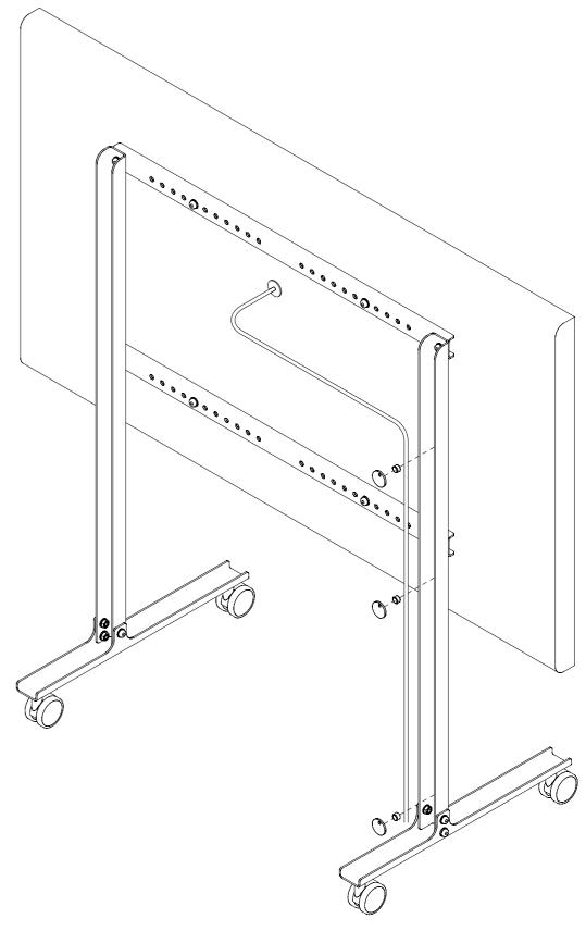
Organize and hide your cables along the brackets and the legs of the stand with the included magnets and cable dots.
