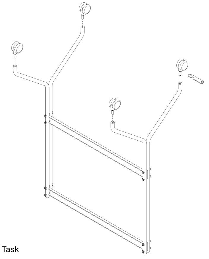
Mount the four wheels into the bottom of the feet as shown. One wheel on each foot. Tighten all connections.
