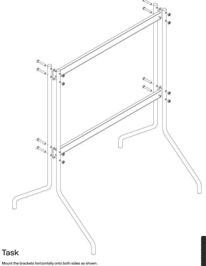
Mount the brackets horizontally onto both sides as shown. Tighten all connections.
